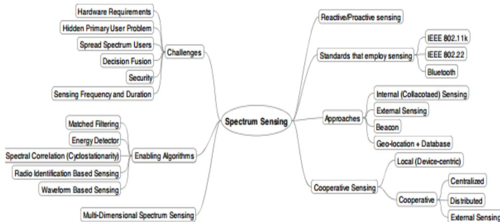
Figure 2: Various Aspects Of Spectrum Sensing For Cognitive Radio.[4]
